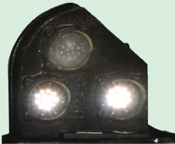
Position type Shunt Signal
