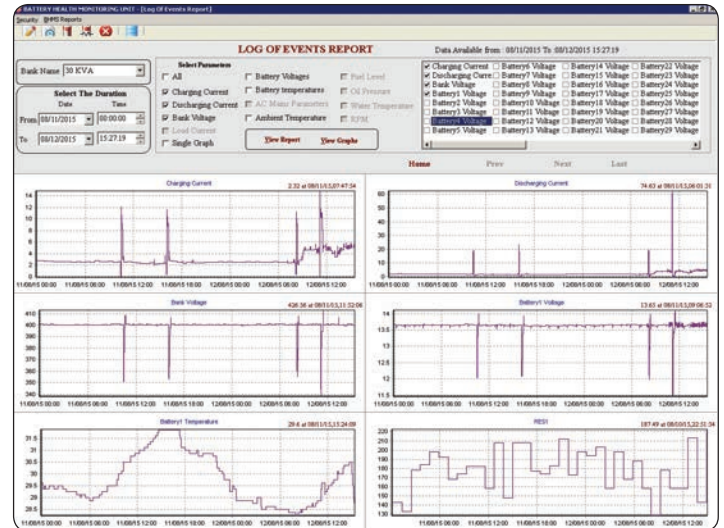
Graphical representation of Bank parameters, Battery / Cell parameters at a glance
